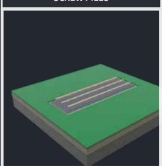
Screw the screw piles into the ground. Attach horizontal joists to the screw piles. Ask an expert which screw piles are suitable for your ground type.
