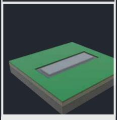
Cast a concrete base for the module set. Make sure that the concrete base is flat.
