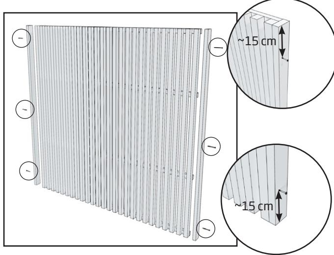
1. Attach filler pieces to sides of the garden screen with 3 screw (4,2 x 55 mm) per piece. Leave the outermost screws about 15 cm away from the edges to prevent cracking.
