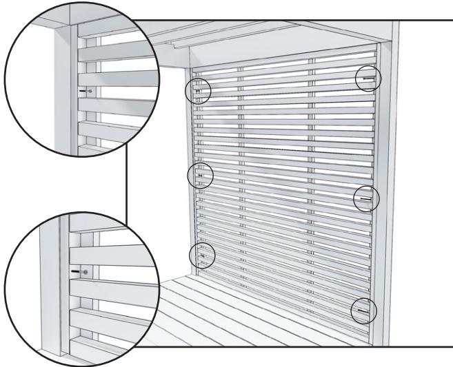
2. Attach with 3 screw (4,2 x 75 mm) per side from the back of the pergola. There will be small gap between the garden screen and the deck of the pergola.
