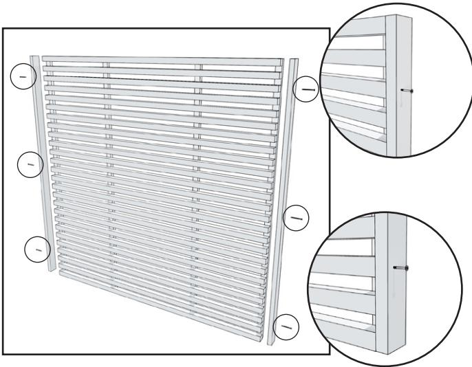
1. Attach the filler pieces to the slats on the sides of the garden screen with 3 screws (4,2 x 55 mm) per piece. Attach the outermost screws to the third slat counted from the top and bottom.
