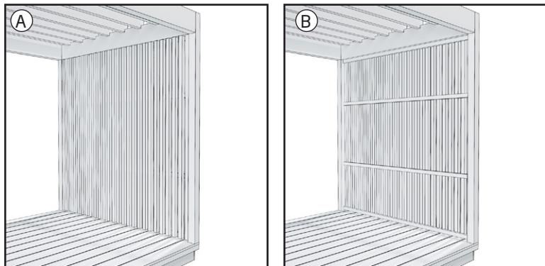
It is also possible to install the garden screen so that the battens binding the wall are on the visible side.
