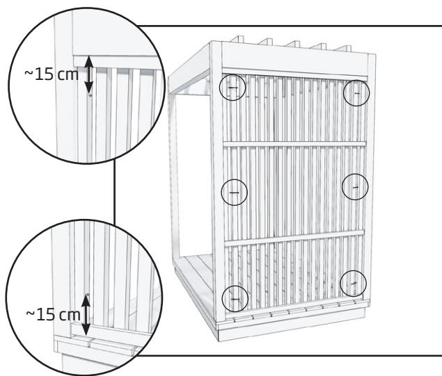
1. Attach the garden screen to both sides of the pergola vertical posts with three (4.2 x 75 mm) screws each, screwing them in from the outside of the pergola. There will be a slight gap between the privacy screen and the pergola deck.
