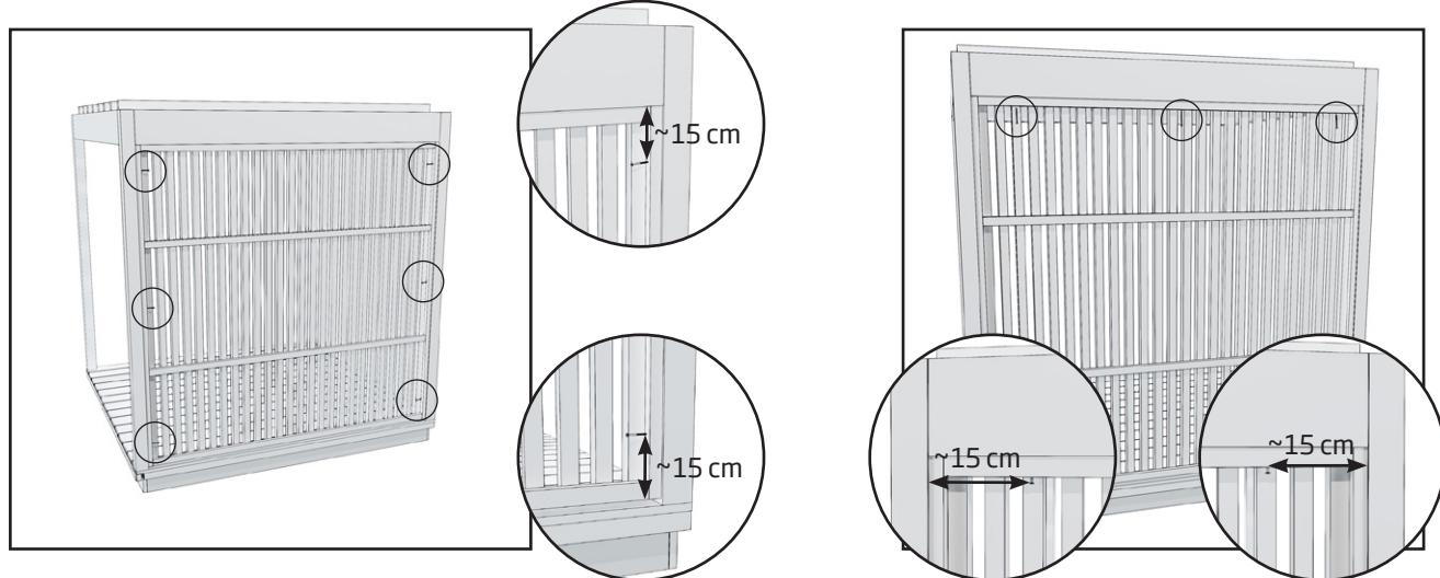
2. Attach the garden screen to both sides of the pergola vertical posts with three (4.2 x 75 mm) screws each, screwing them in from the outside of the pergola. There will be a slight gap between the privacy screen and the pergola deck.
