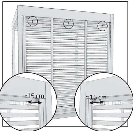
3. Attach with 3 screws (4,2 x 75 mm) to the top.
