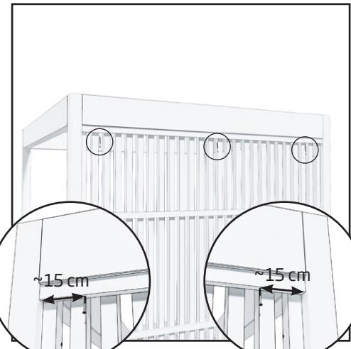
1. Attach the garden screen to both sides of the pergola vertical posts with three (4.2 x 75 mm) screws each, screwing them in from the outside of the pergola. There will be a slight gap between the privacy screen and the pergola deck.
